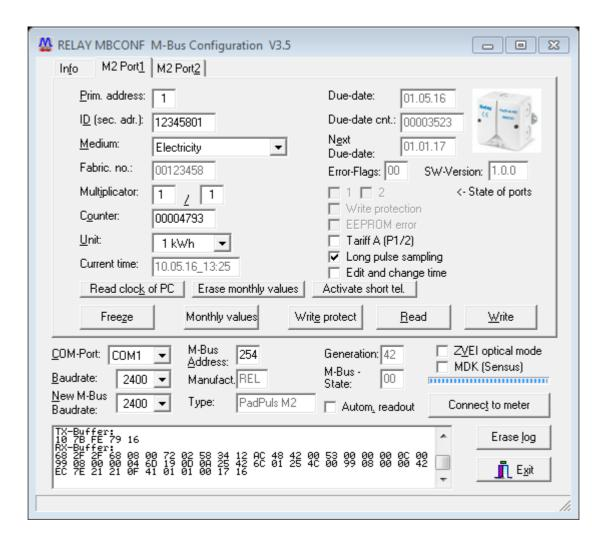
This sheet shows the current settings and values of the respectively pulse channel (port) of the PadPuls M2 (in this example: Port 1 in the mode "long telegram"). The following input boxes and buttons are used to change the parameters of the pulse adapter:
