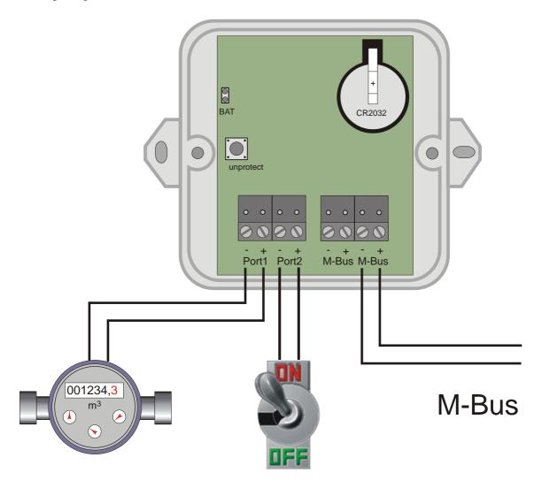
The tariff mode can be activated with the configuration software MBCONF. You are using this operating mode to adopt a meter with two tariffs supplying just one joint pulse output and a tariff switch signal to the M-Bus. Port1 is the pulse input and Port2 is the tariff switch. The PadPuls counts the incoming pulses to channel 1 while the input at channel 2 is open and to channel 2 while the input at channel 2 is closed.
