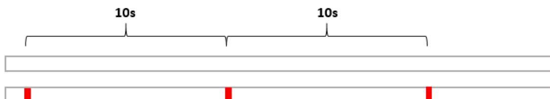
Figure 2: Soft start LED indication
