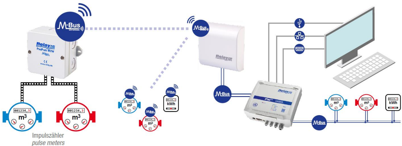
Picture: Wireless M-Bus System with PadPuls M2W, wM-Bus / M-Bus Gateway RelAir R2M and PW250
