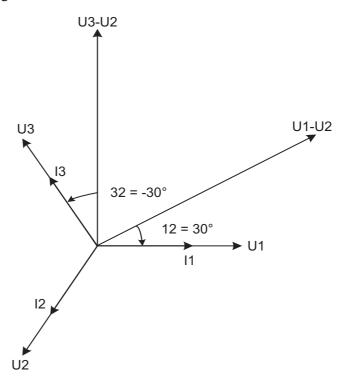
a pure resistive load where the phase currents are in phase with its respective phase voltages.
